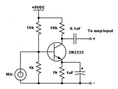
The following schematic is similar, except it is designed for high impedance, crystal type microphones (10,000 or greater).
