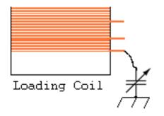
The biggest drawback with a variable capacitor is that it can be hard to find them (your best bet is at HAM fests and old electronic parts stores). Also, after about 10 Watts they have to be high voltage or else they won't work (the RF electricity will arc across the capacitor's metal plates). If you run into this problem or can't find a suitable variable capacitor, an alternative is to use a variableinductance method of fine-tuning, such as a variometer.
