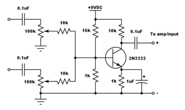
The following circuit is for high impedance microphones:
