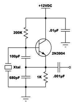
I have had extremely good luck with this circuit in transmitters. It works well, and puts out a very clean powerful signal for the buffer amplifier stage. Drift is nonexistent.
