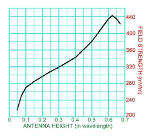
To a point, increasing the length of a vertical radiator will increase the efficiency of the antenna. Note that peak signal strength is reached at 5/8. Despite being the optimal point for signal strength, it is not the optimal point for vertical antennas, as it is accompanied by a high angle of radiation (not visible in graph). This is undesirable, because it leads to skywave interference and a reduction of the groundwave.
