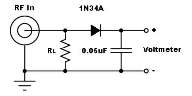
RL is the load resistance, either a dummy load or a tuned antenna. If you know the load resistance, you can find the power and current:
