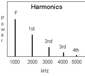
Harmonic interference is the worst type of interference, because it exists on all transmitters and is strong. Mathematically, a harmonic is a signal that appears on every multiple of the transmitter's output frequency. For example, an LPAM transmitter operating at 1650kHz would generate the first harmonic at 3300kHz and the second at 6600 kHz. This signal can be quite strong, sometimes as much as half the power of the operating frequency output. There are many harmonics, but the
